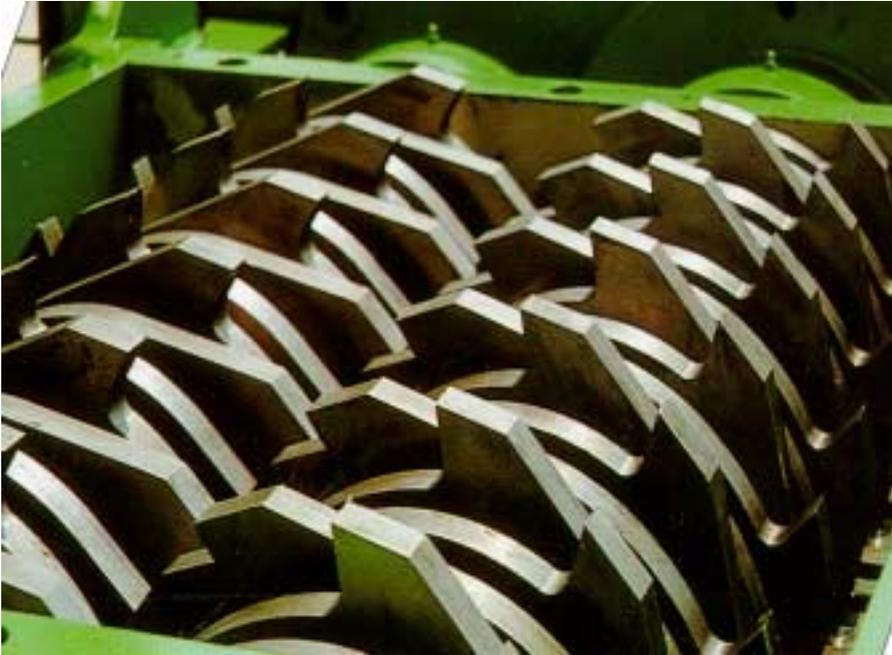
**Depending on the size and nature of the composite, a pre-shredding to a particle size of approx. 30 mm is carried out in one or more operations.**
