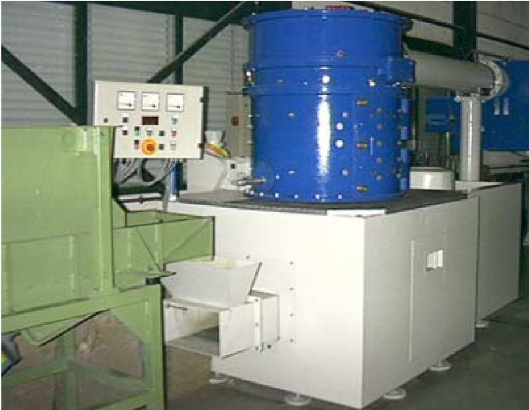
**The pre-shredded material is fed by a dosing unit to the accelerator where it is then delaminated.**
