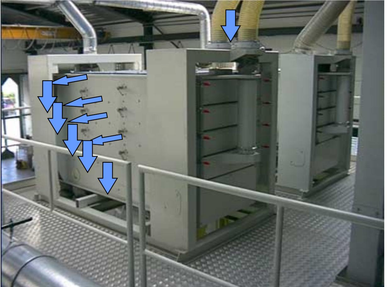
**In various sieve layers the delaminated material mix is separated according to size.**
