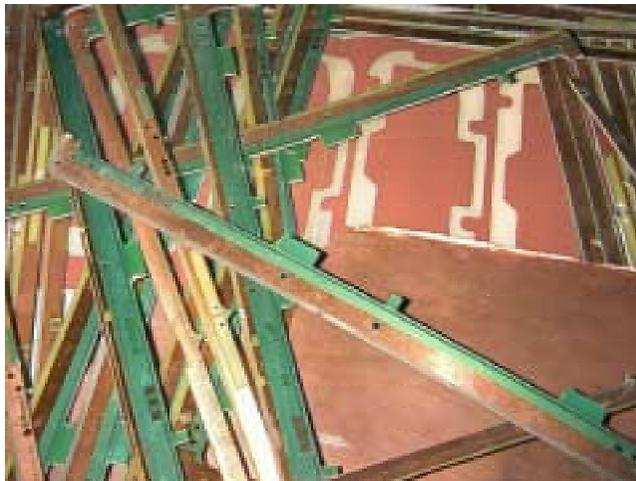
**In the manufacture of products e.g. printed circuit boards, cuttings of copper and glass fibre epoxy composite material waste arise.**
