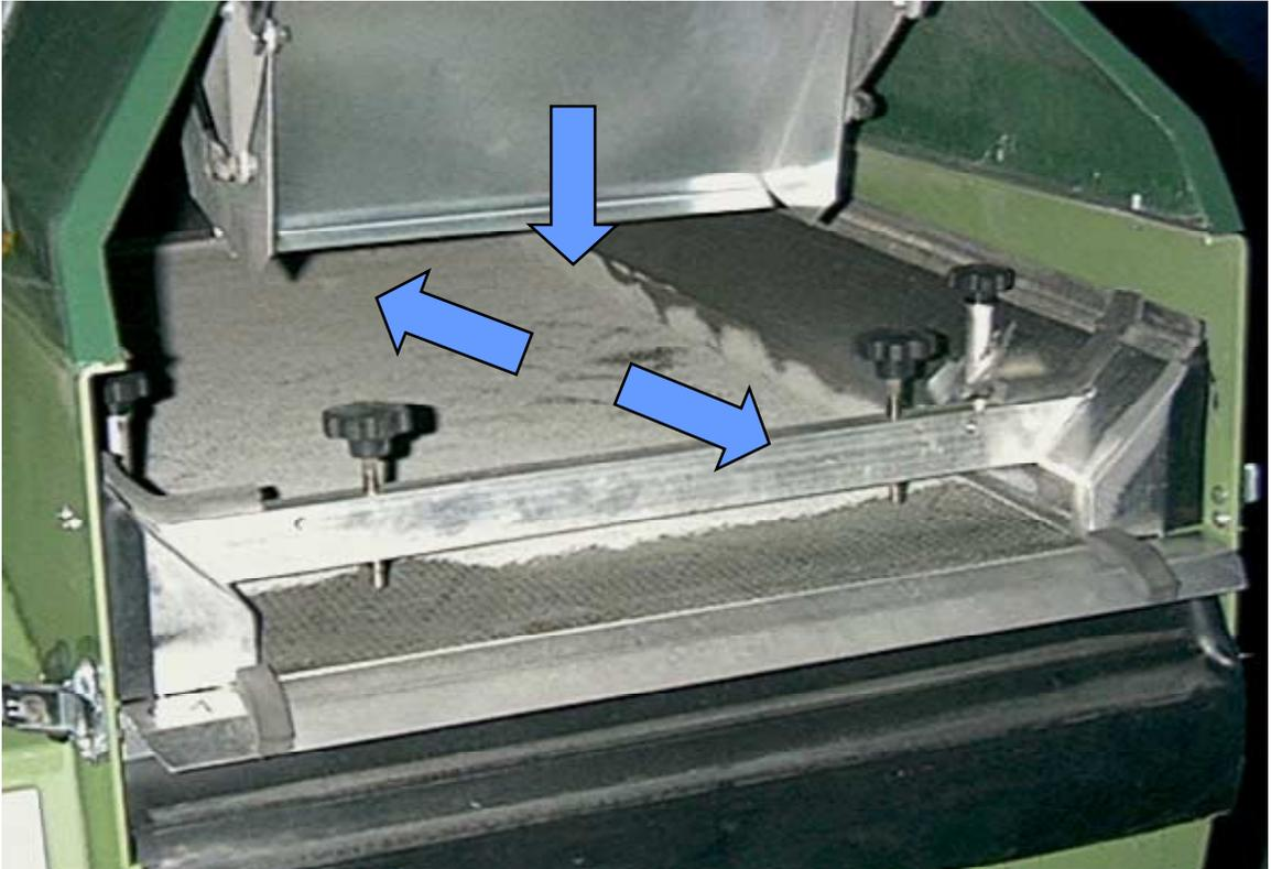
After sieving, the fractions are then separated into single components according to weight and structure.
